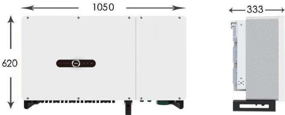
Fig 2-4 Inverter Dimensions
