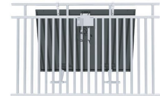
Attaching the inverter to the railing using stainless steel ties
