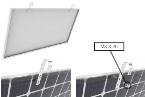
4.12 The hook and railing connection: the hook hangs on the balcony railing, through the bolt to prevent it from falling out;
